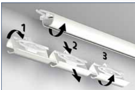
Ceiling click bracket mounting process
